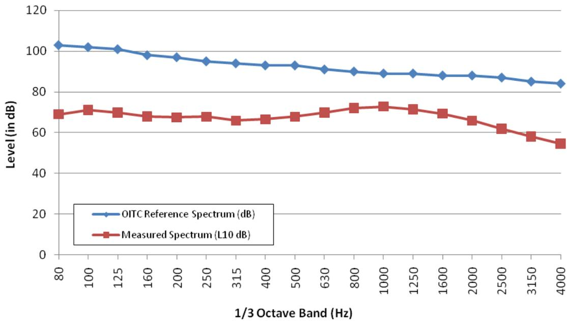
Fig. 4 – Measured vs. OITC Reference Spectrum
