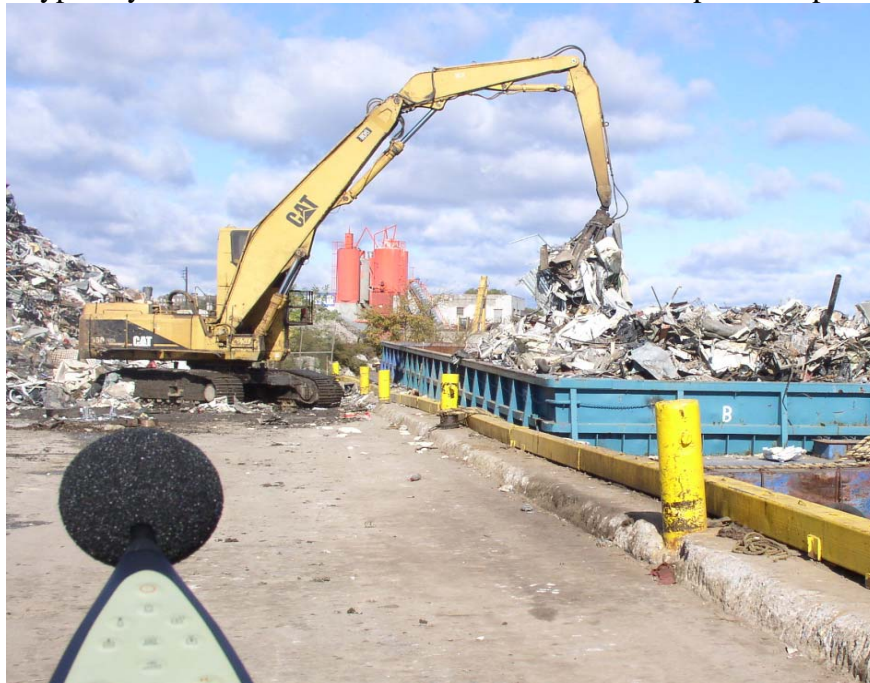
Figure 1: Measuring a crane loading scrap metal into a barge with a B&K 2260 SLM (lower left).
